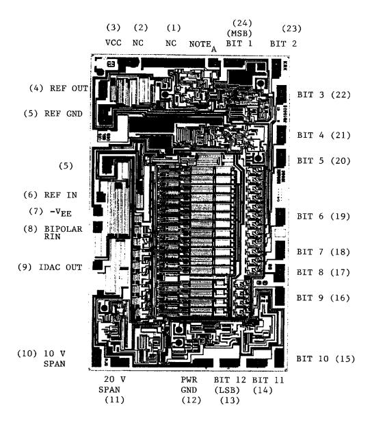
Note: Pad numbers reflect terminal numbers when placed in case outlines J and X (see figure 1).
