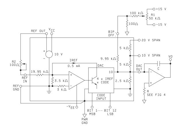
FIGURE 2. Calibration circuit, unipolar voltage output.
