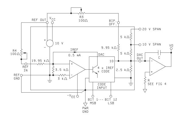
FIGURE 3. Calibration circuit, bipolar voltage output.
