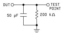
FIGURE 4. Load circuit and switching waveforms.
