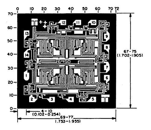
NOTE: Pad numbers reflect terminal numbers when placed in case outlines C and X (see figure 1).
