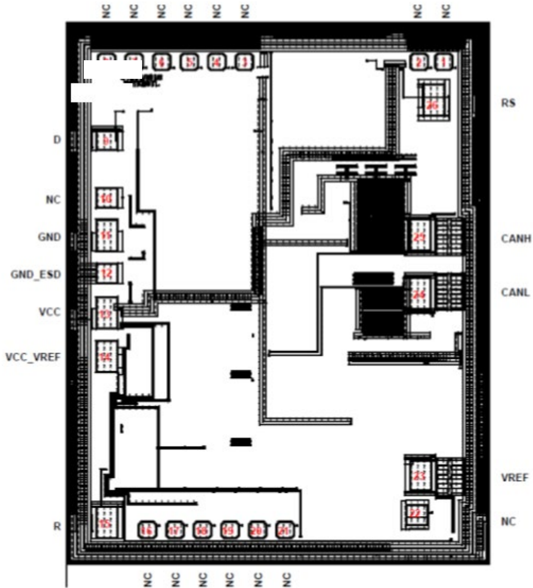
FIGURE A-2. Die bonding pad locations and electrical functions.
