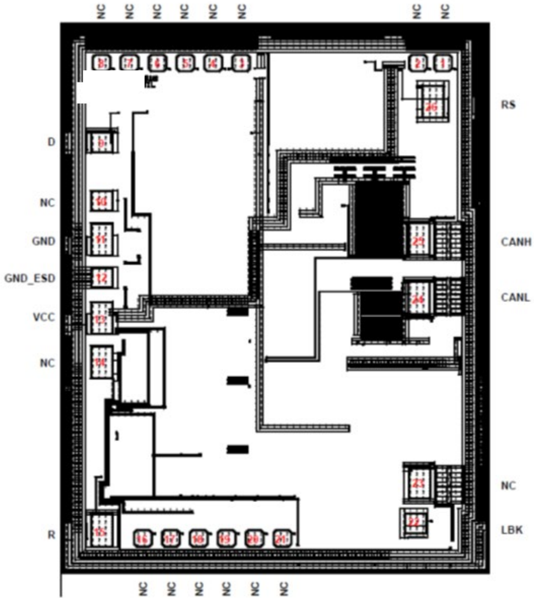
FIGURE A-1. Die bonding pad locations and electrical functions.
