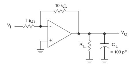
FIGURE 6. Gain of 10 inverting amplifier.
