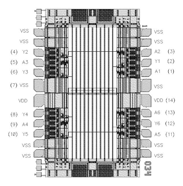
Note: Pad numbers reflect terminal numbers when placed in Case Outlines C and X (see Figure 1).
