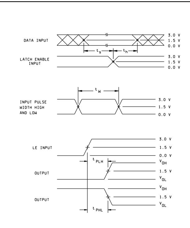
FIGURE 5. Switching waveforms and test circuit.
