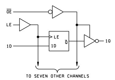
FIGURE 3. Logic diagram.
