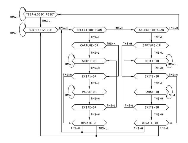
FIGURE 4. Test access port controller and scan test register.
