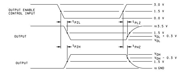
FIGURE 6. Switching waveforms and test circuit.
