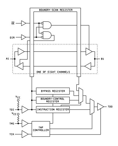
FIGURE 3. Block diagram.
