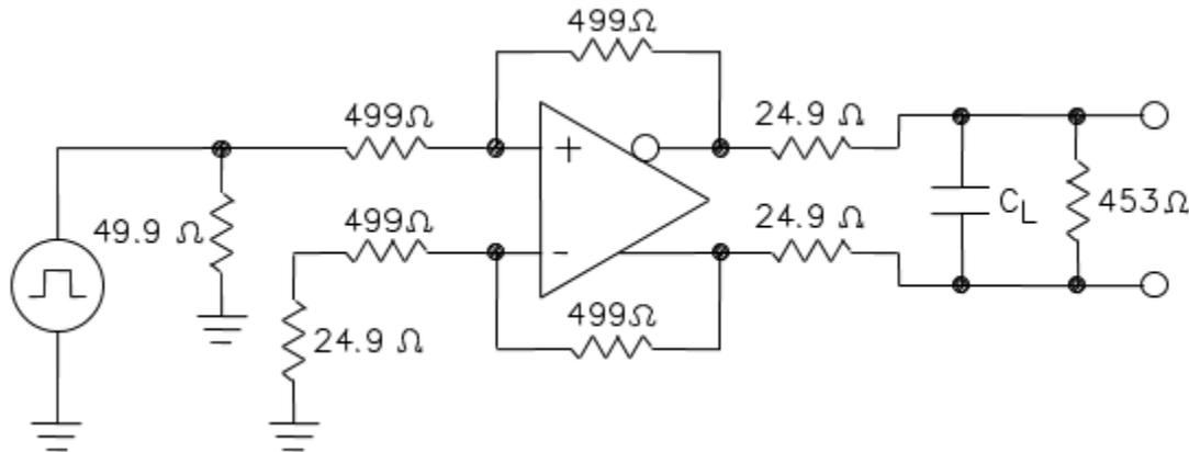
FIGURE 3. Driving capacitive load application.
